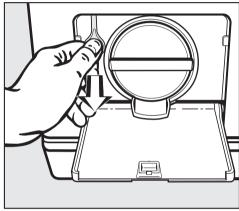
Pull the emergency release downwards until the machine outer lid opens.
